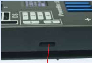
Socket for Multiplex MSB telemetry
