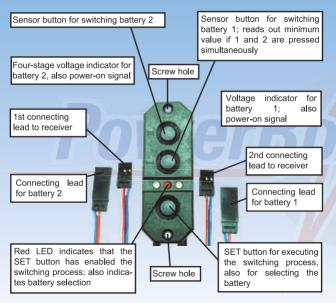
The switch is designed to be installed in the model using a pair of screws (supplied) fitted through the two countersunk holes.
