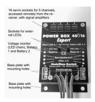
The two receiver batteries are connected via the pair of integral high-current sockets. In theory the PowerBox 40/16 will also work with a single battery, but this forfeits the extra security of a dual-battery power supply.
