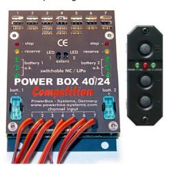
Double voltage stabilisation with linear regulation and double battery monitor, double signal amplification for each channel, twin electronic safety switches (SensorSwitches) petty patent no.: 203 13 420.6
