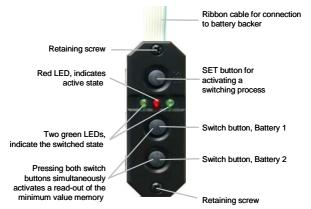
The **SET** button is slightly recessed, and its purpose is to prepare and carry out a switching process. Holding the **SET** button pressed in "arms" (activates) the switches: after about one second the red LED lights up. This indicates that the electronic switches are armed, and ready to be switched.
