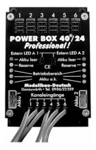
With seven servo signal amplifiers, two independent voltage monitors and regulated receiver power supply
