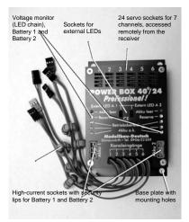
The two receiver batteries are connected via the pair of integral high-current sockets. In theory the PowerBox 40/24 Professional will also work with a single battery, but this forfeits the extra security of a dual-battery power supply.
