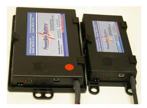
These LiPo batteries currently represent the safest, most reliable battery packs available, as they contain a balancer and a low-voltage monitor as well as complete charge and security electronics.
